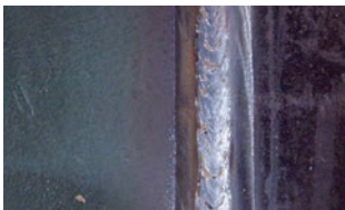
One of the primary contributors to De-Cal's success has been the conversion of most root pass applications to the Miller RMD process. A root pass using the process is shown here.
