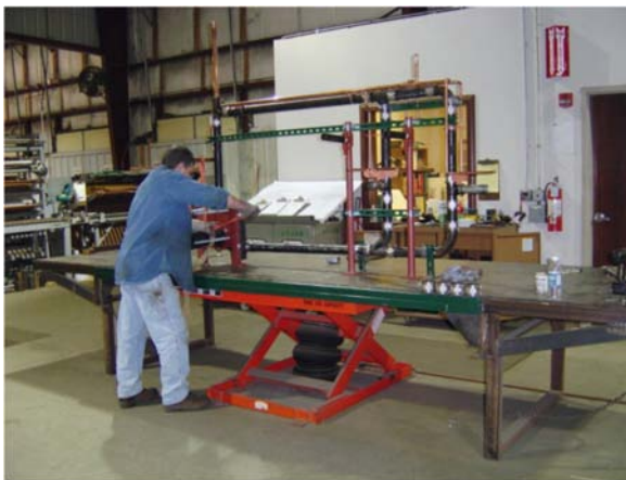
Using a lift table can enable one man to work at the correct working height. Photo courtesy of P1 Group.
