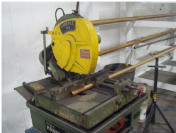
Simple chop saw set up with jacks for cutting copper pipe.
