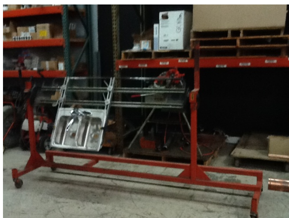
This fit out jig can be rotated to attach trim pieces to both the top and bottom of the sink.
