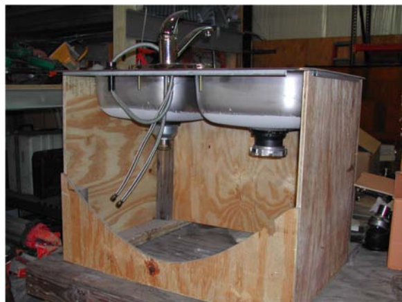
Plywood jig built to handle a double sink. Photo courtesy of CFI Mechanical.
