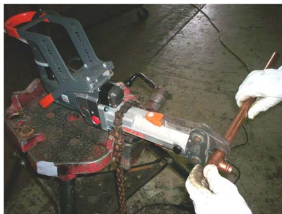
Pre-fabrication shop ingenuity. This contractor mounted a ProPress tool for two-handed control.
