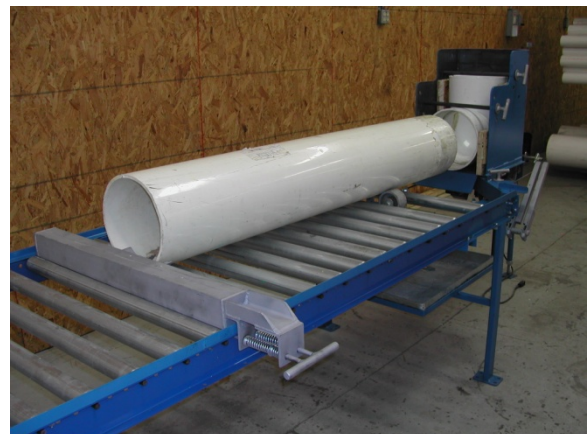
This jig assists plumbers in pushing together large bore PVC.
