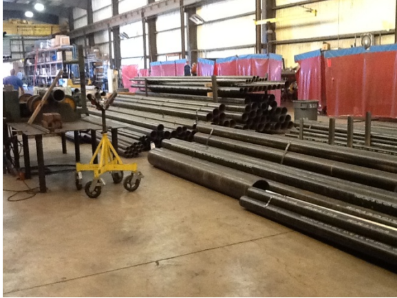
Avoid storing pipe in a production area.
