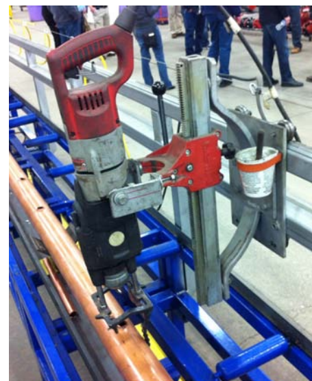
SA Communale built this T-Drill press capable of handling 20' Lengths of copper in various sizes.
