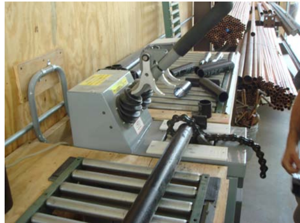
Hydraulic pipe cutters can snap pipe 1 1/2" to 6" in seconds. Photo courtesy of CFI Mechanical.
