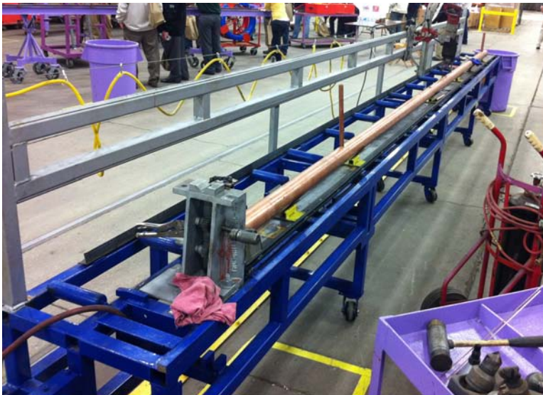
SA Communale built this T-Drill press capable of handling 20' Lengths of copper in various sizes.
