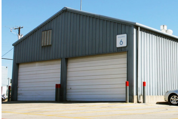
Grade level doors allow for the movement of materials without truck wells, which take away valuable floor space.
