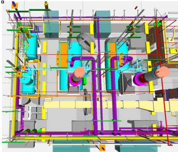
As electronic drawings become more accurate, more possibilities are open to pre-fabrication.
