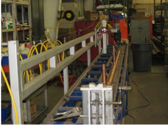
Custom-built machines like this tee-pulling station take training on operations and safety for all new workers. Photo courtesy of SA Commune.
