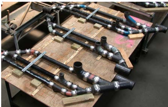
A jig allows many similar pipe configurations to be assembled in less time.
