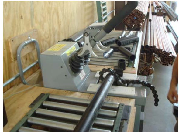
Automatic pipe snappers allow for quick clean breaks in under a minute. Photo courtesy of CFI Mechanical.
