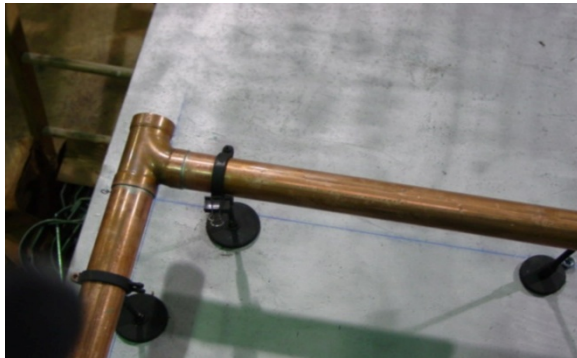
This jig table includes a sheet of galvanized metal. After a chalk line is snapped on the table to plot the design, magnetic fasteners hold the pipe. A simpler version can be built with a sheet of plywood and spring clips.
