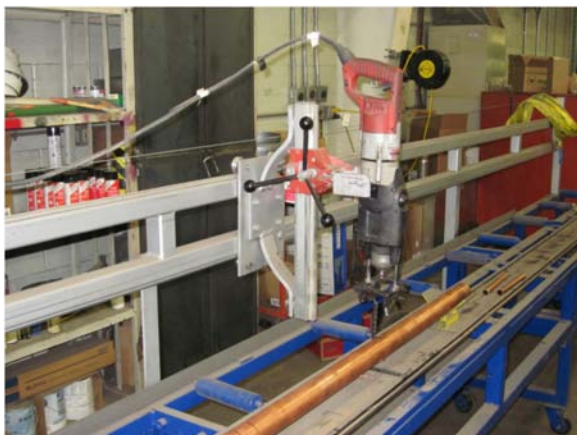
Custom tool applications like this tee drilling station are great for productivity in the shop, but impractical in the field. Photo courtesy of SA Commune.
