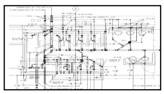
Step 3. - Once the shop drawings are approved, generate individual spool drawings and release them to the fabrication shop for production.
