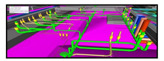
Step 2. - Once the BIM Model is signed off, generate shop drawings and submit to the Mechanical Engineer of Record or the owner/client for approval.
