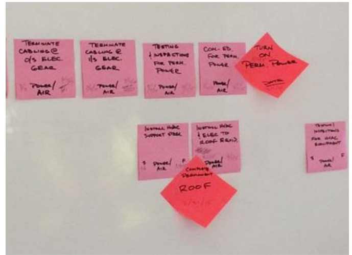
Figures 4 and 5 are examples of a “mini” pull production schedule developed during a stand-up session between an electrical contractor and mechanical contractor to determine, step-by-step, what needs to be executed to establish permanent power to air handler units.
