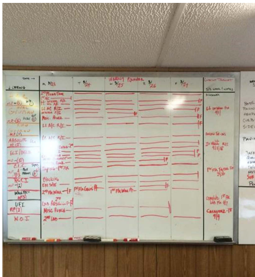
Figure 8 and 9. Weekly work plans are best executed on a whiteboard located on the jobsite but can also be maintained in other forms. Again, form should follow function.
